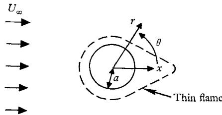
FIGURE 1. Co-ordinate system for flow past a spherical droplet.
