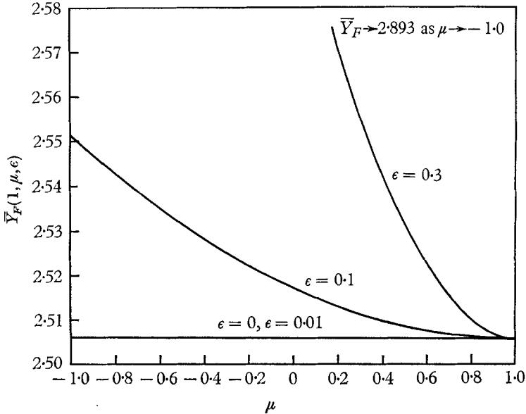
FIGURE 3. Variation in the stoichiometrically adjusted mass fraction of fuel  $\bar{Y}_F$  with angle at the droplet surface.
